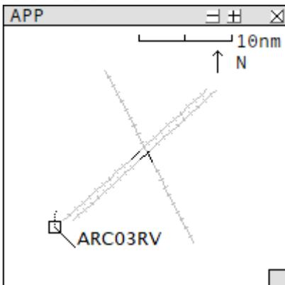
The Approach Window displays traffic around the airport (traffic on the ground at the airport is hidden). The window displays the runway centerlines, and optionally extended centerlines and various maps.
