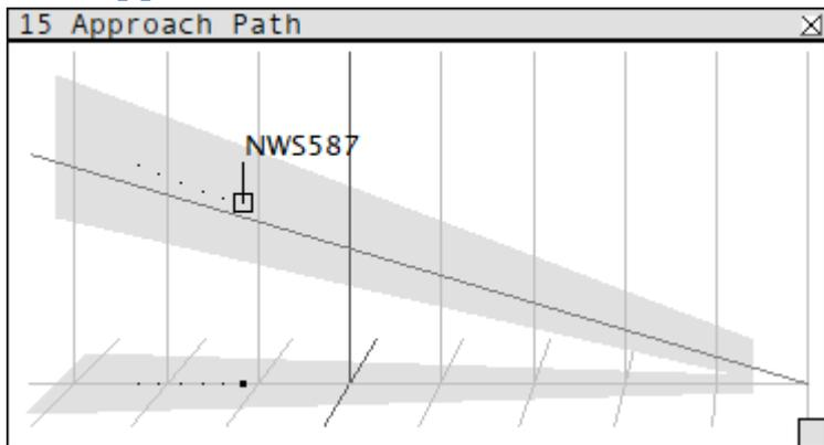
The Approach Path Window displays a vertical and horizontal view of a pre-defined approach. Distance lines are shown at 1 nm intervals.
